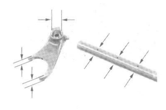
Check the shaft for scratches, scoring or evidence of insufficient lubrication.
