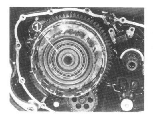
One-way clutch/clutch center B assembly
