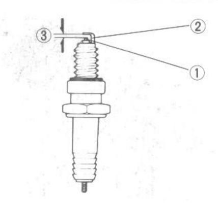
(1) Center electrode (3) Spark plug gap
