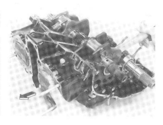
Push the connecting rods and piston out through the top of the cylinder bores.
