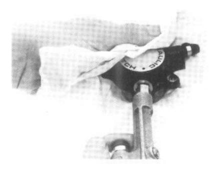
Remove the piston from the cylinder. If piston removal is hard, place a shop towel over the piston to cushion the piston when it is expelled, and position the cylinder with the piston down.
