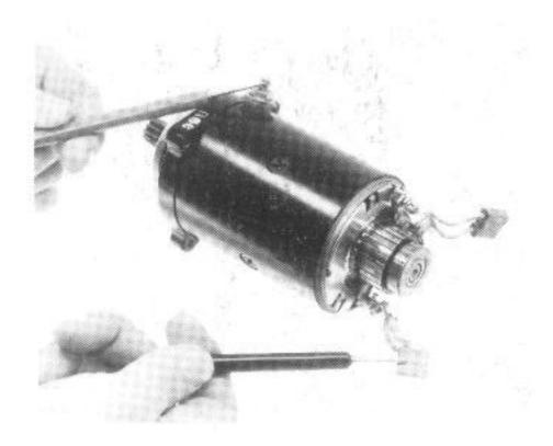
Check for continuity from the cable terminal to the motor case.
