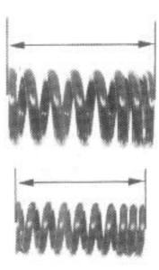
Measure the free length of the inner and outer valve springs (page 214).
