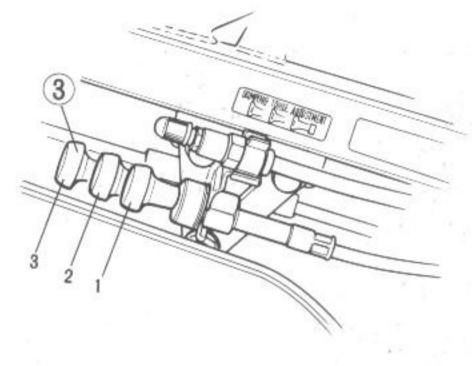
(3) Shock absorber damping adjuster
