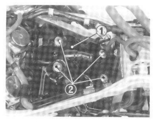
Tighten the cylinder head and camshaft holder bolts in a criss-cross pattern in 2-3 steps.
