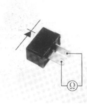
Check for continuity with an ohmmeter.
