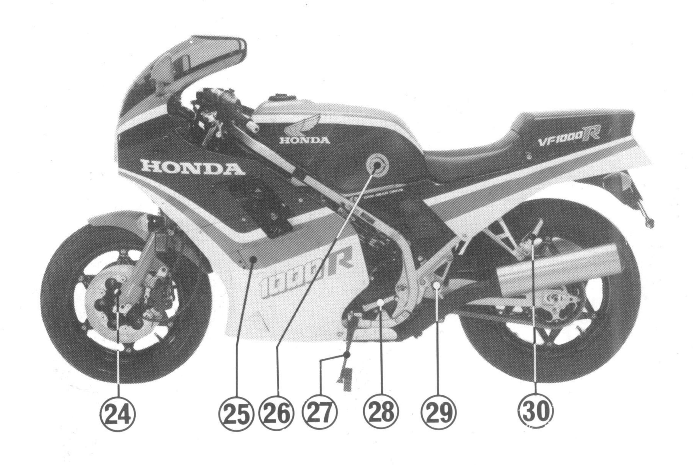
(24) Anti-dive damper adjuster (25) Air intake lid (26) Fuel valve
