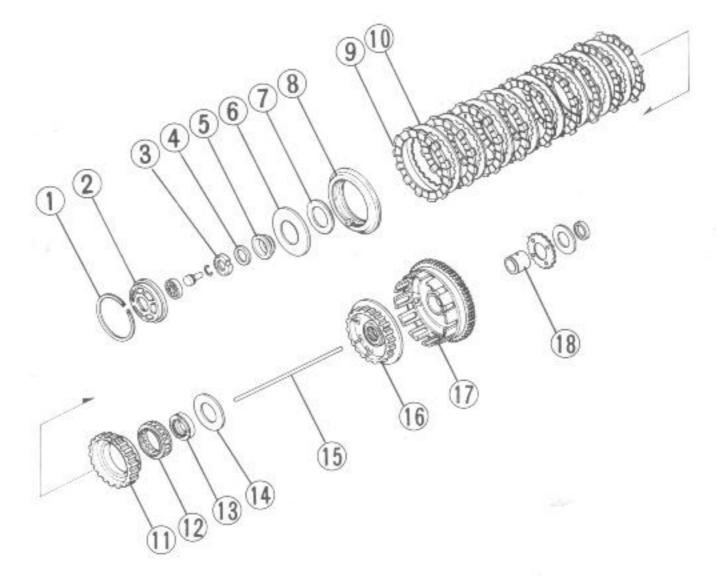
Remove the clutch spring set plate, clutch spring and washer.
