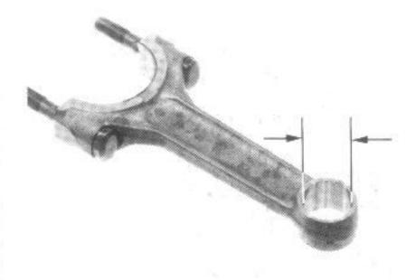
Measure the connecting rod small end I.D. (page 216). If the reading exceeds the service limit, replace the rod (page 122).
