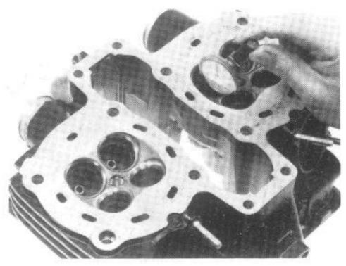
If the stem-to-guide clearance exceeds the service limits with new guides, replace the valves.
