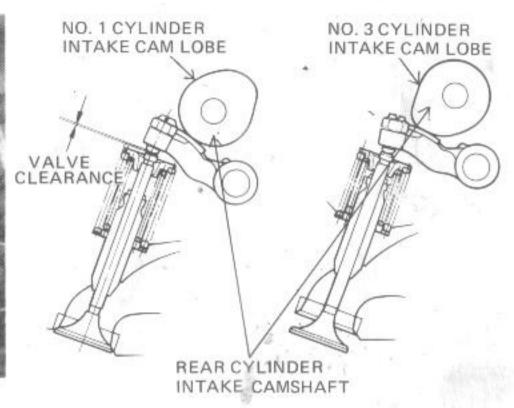
To inspect the No. 1 cylinder intake valves, rotate the crankshaft counter-clockwise so that the No. 3 cylinder intake valves are at maximum lift.
