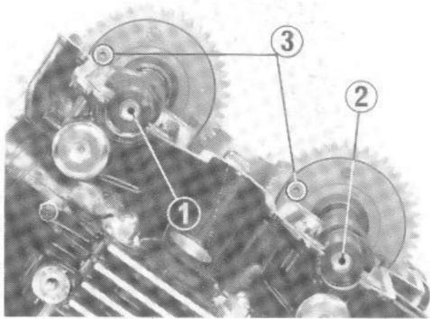
(1) Rear cylinder intake camshaft
