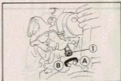
(1) Throttle stop screw (A) Increase (B) Decrease
