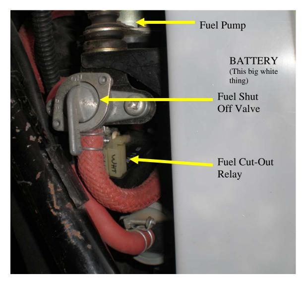
To get the Fuel Cut-Out Relay out of there, I had to remove the left side fuel pump mounting bolt, which also holds the Fuel Shut Off valve mounting bracket. Then I dropped the bracket down and left the bolt in place. Then I could pull out the Fuel Cut-Off relay. See below:
