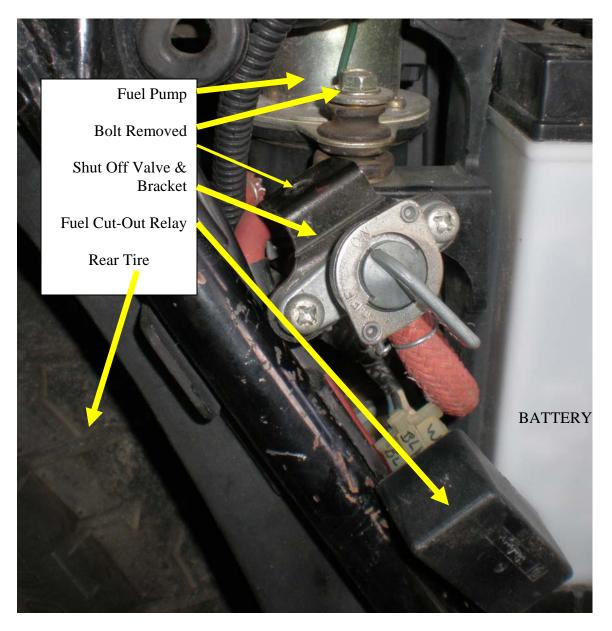
Note that from this view, the wires are (Left to Right) Blue, Black, White. (Ignition, +12 Volts, Output)
